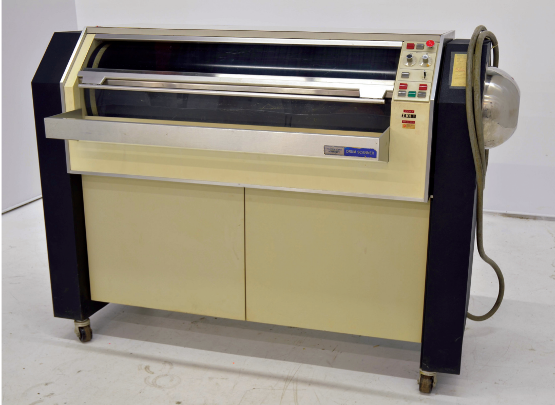
Figure 2: This scanner was developed by International Business Machines (IBM) for the Canada Land Inventory. It converted graphic information to digital format, an essential step in relation to the Canada Geographic Information System. The scanner is now part of the Ingenium (Canada's Museums of Science and Innovation) collection. IBM Scanner, 1963, Artifact No. 1986.0821
