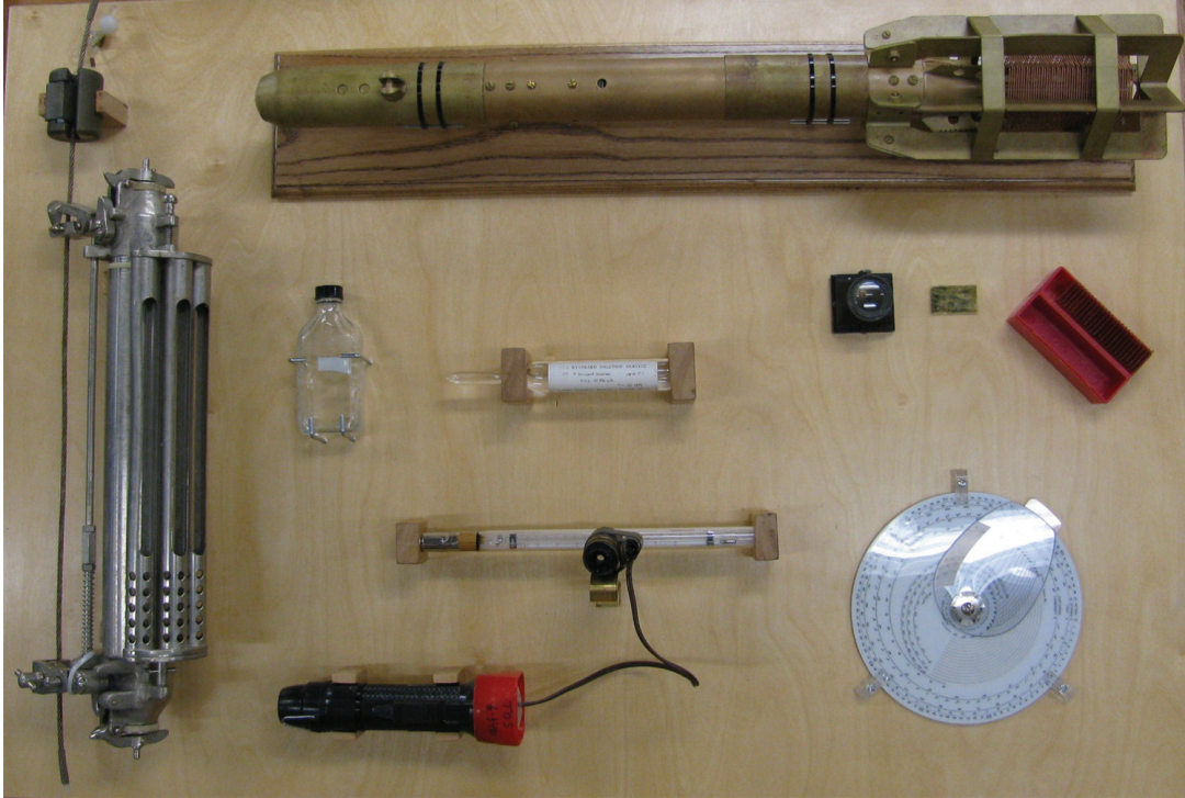
Figure 1. Tools of the trade for physical oceanography in the early 1960s. From the top: bathythermograph (BT) for measuring water temperature at various depths; slide holder and glass magnifier for reading slides from the BT; special slide rule for converting thermometer readings to temperature and depth; illuminated magnifier for reading reversing thermometers; just above is a reversing thermometer; above that is a standard sample of sea water used to compare recovered samples; to its left is a sterile water bottle for storing seawater samples for later testing; far left is a Knudsen water bottle for collecting seawater samples. Credit: BIO Oceans Association, Physical Oceanography - Twentieth Century Tools of the Trade, http://www.bio-oc.ca/phys_oc/index.html downloaded Feb. 25, 2014.
