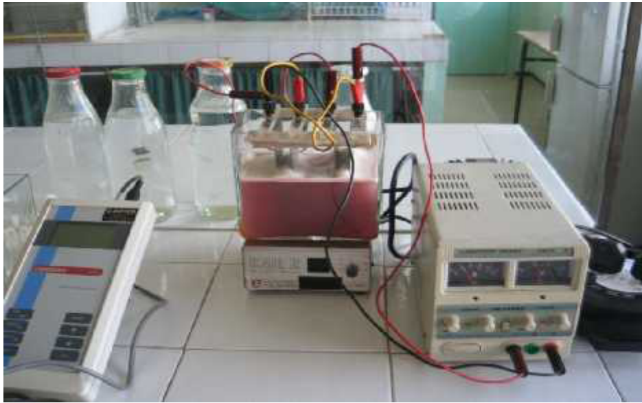
Figure 1. Dispositif d'électrocoagulation. Electrocoagulation device.
