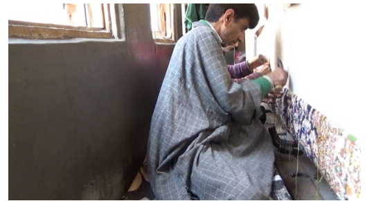
Figure 4 In KCW, weavers sit on backside of the loom while lower rollers point towards the other side. In ACW (figure 3), weavers sit on the side facing the rollers.
