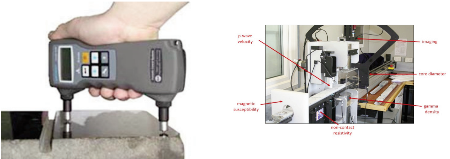
Figure 5. Left: example of hand-held measurement of drill core sonic velocity. Right: example of a Geotek multi-sensor core logger used for collecting petrophysical measurements (e.g. gamma density, p -wave velocity, resistivity, magnetic susceptibility, etc.) from drill core.
