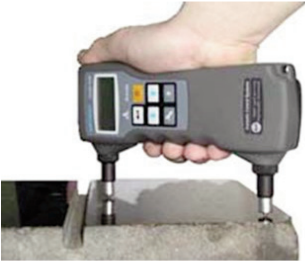
Figure 5. Left: example of hand-held measurement of drill core sonic velocity. Right: example of a Geotek multi-sensor core logger used for collecting petrophysical measurements (e.g. gamma density, p -wave velocity, resistivity, magnetic susceptibility, etc.) from drill core.
