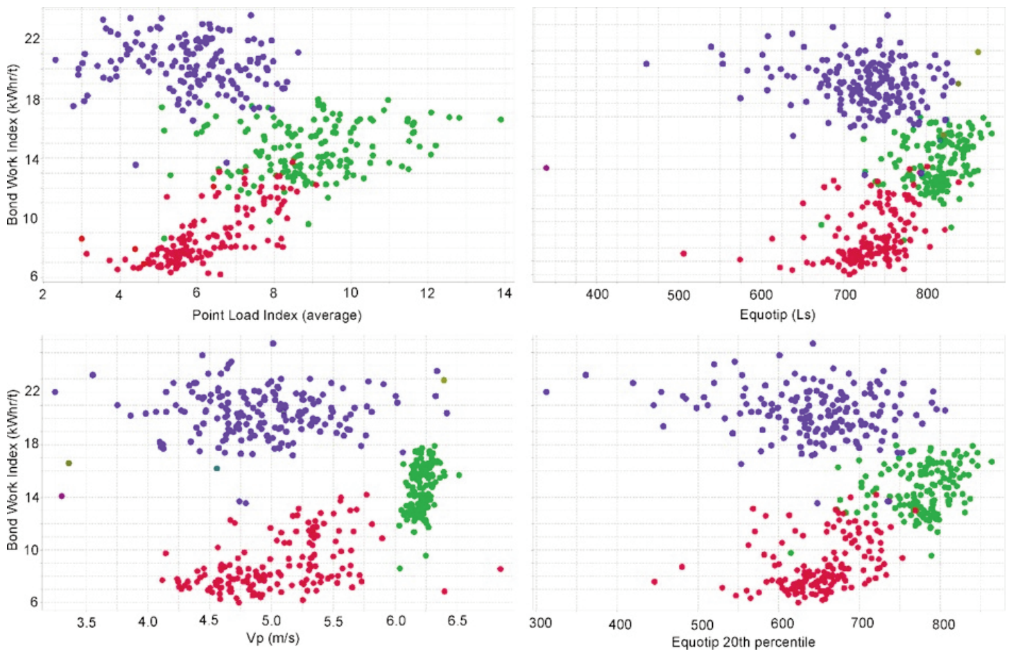
Figure 8. Comparison of small scale tests with Bond Work index (BMW i ) for a range of deposits in the AMIRA P843A database. V_p is compressional seismic velocity. Equotip (i.e. rebound hardness) results reported by Leeb hardness value (Ls; Proceq: https://www.proceq.com/compare/equotip-portable-hardness-testing/ ) and 20 th percentile of 100 individual Equotip readings over 2 m intervals. Each colour represents a different deposit style as in Figure 7.
