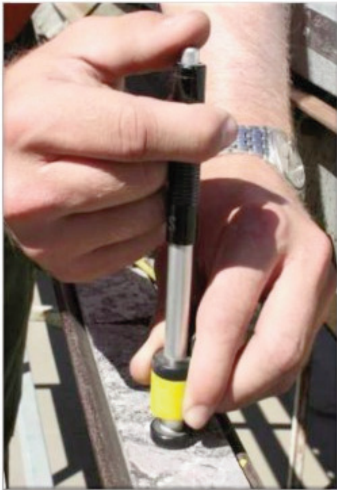
Figure 5. Left: example of hand-held measurement of drill core sonic velocity. Right: example of a Geotek multi-sensor core logger used for collecting petrophysical measurements (e.g. gamma density, p -wave velocity, resistivity, magnetic susceptibility, etc.) from drill core.
