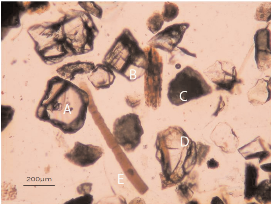
Figure 2. Characterization of mineral particles in house dust by polarizing light microscopy: A) garnet, B) orthopyroxene, C) lithic fragment, D) K-feldspar, and E) segmented insect antenna (pers. comm. 2008, M. Woldemichael, Department of Earth Sciences, University of Ottawa).
