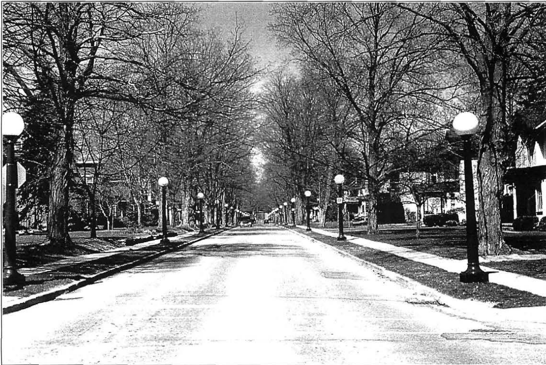
Figure 10: This is the view looking north along Lansdowne Street North from Salisbury Avenue. The original lampposts were made of iron and steel and weighed 450 pounds. The City of Cambridge replaces them as they wear out with custom-moulded aluminum ones weighing 150 pounds. The trees in this elite area need not be trimmed, as all electrical and telephone wiring is located along rear alleys. No driveways interrupt the streetscape, as vehicular access is also gained through these alleys. Photo: John S. Hagopian, 1998.
