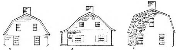
FIGURE 4. Types of gambrel roofs: (A) New England; (B) Dutch; (C) Swedish (Philip White). "Types of Gambrel Roofs," illustration from Hugh MORRISON, Early American Architecture (New York, Oxford, 1952).
