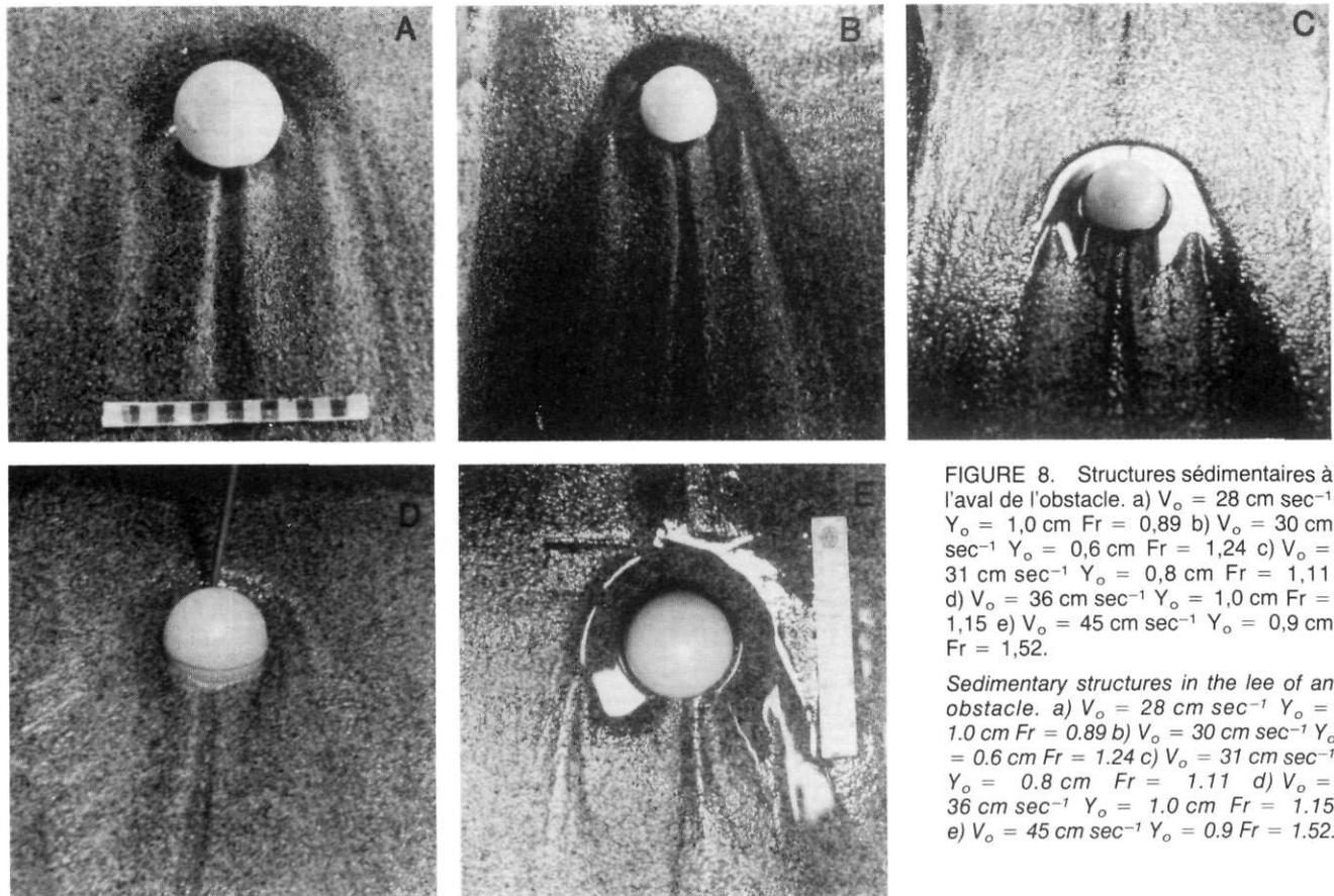
FIGURE 8. Structures sédimentaires à l'aval de l'obstacle. a)  $V_o = 28 \text{ cm sec}^{-1}$   $Y_o = 1,0 \text{ cm}$   $Fr = 0,89$  b)  $V_o = 30 \text{ cm sec}^{-1}$   $Y_o = 0,6 \text{ cm}$   $Fr = 1,24$  c)  $V_o = 31 \text{ cm sec}^{-1}$   $Y_o = 0,8 \text{ cm}$   $Fr = 1,11$  d)  $V_o = 36 \text{ cm sec}^{-1}$   $Y_o = 1,0 \text{ cm}$   $Fr = 1,15$  e)  $V_o = 45 \text{ cm sec}^{-1}$   $Y_o = 0,9 \text{ cm}$   $Fr = 1,52$ .
