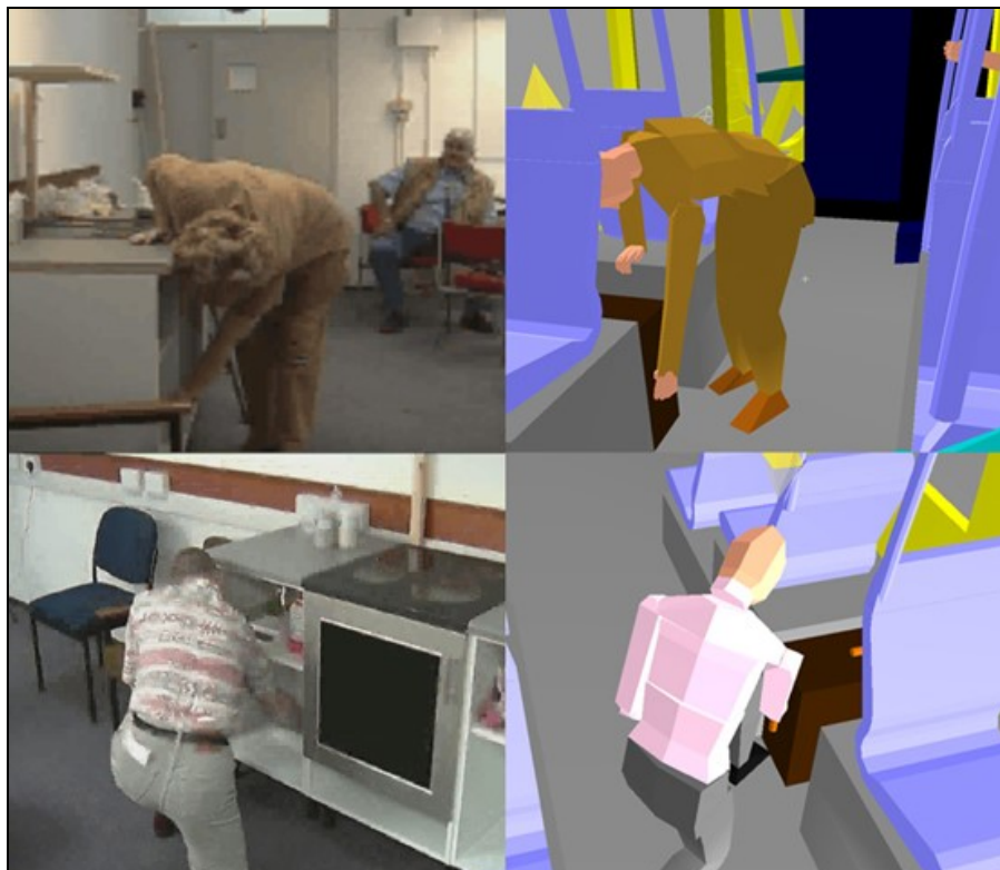
FIGURE 9 : EXAMPLE OF VIDEO STILLS SHOWING POSTURES ATTAINED BY PARTICIPANTS REACHING TO LOW SHELVES ON 'KITCHEN' RIG DURING TRIALS, AND AS SIMULATED IN HADRIAN (FROM MARSHALL ET AL, 2010)
