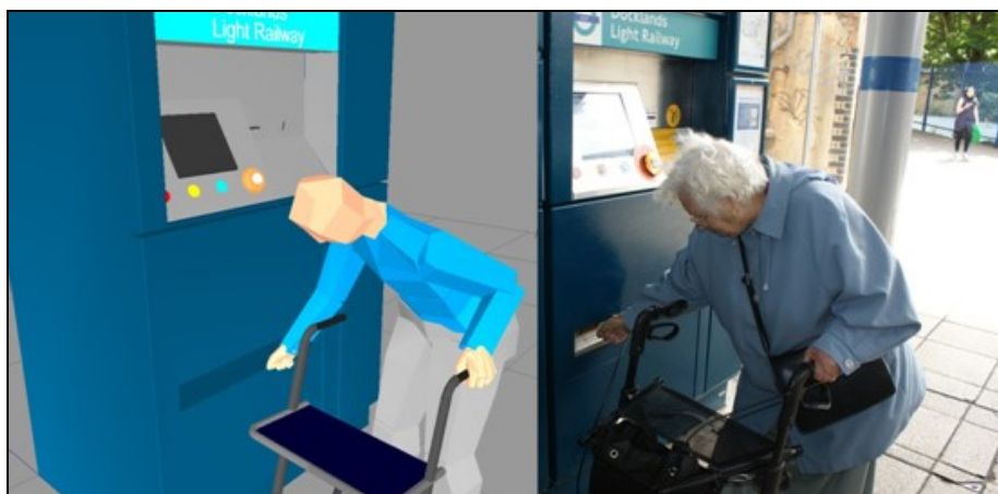
FIGURE 7 : HADRIAN SIMULATION AND REAL LIFE PHOTOGRAPH OF ONE PARTICIPANT ATTEMPTING TO COLLECT THEIR TICKET FROM THE TICKET MACHINE AT GREENWICH DLR STATION
