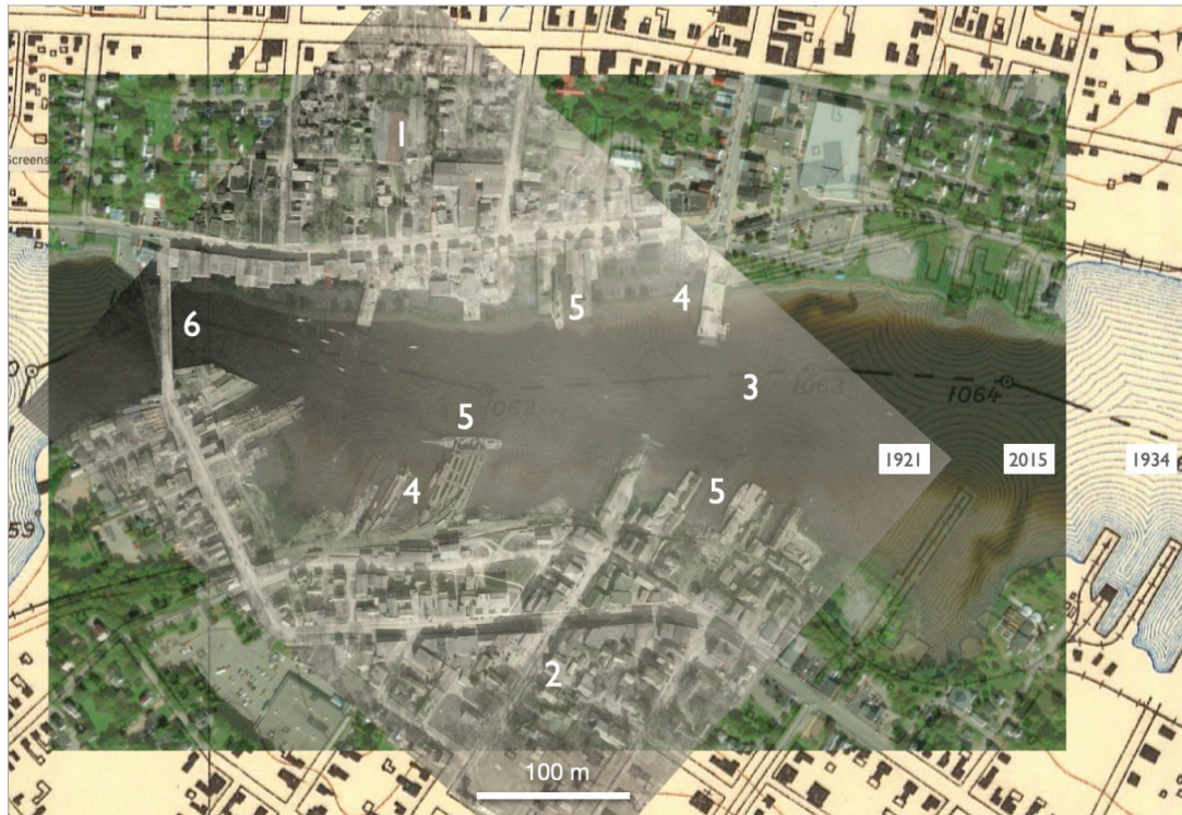
Figure 8. Vertical aerial view of the St Stephen (1) and Calais (2) waterfront area along the St Croix River (3) showing past and present locations of wharf installations (4), berthed vessels (5) and tidewater levels toward the International Bridge (6). The semi-transparent renditions of the 1921 and 2015 imagery are overlaid digitally on the 1934 IBC boundary map of the area. Sources: NAPL (1921 air photo K3-13), IBC (1934 St Croix Boundary Map Sheet 13), IBC – Geo.NB 2015 (Digital Ortho Image St Stephen 24383E73546N)
