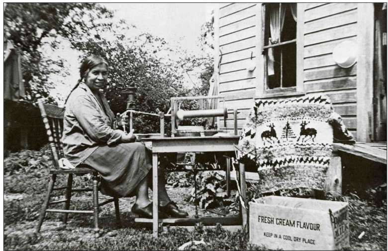
Fig. 7 Mrs. Helen Jimmy spinning wool on a second type of converted treadle sewing machine with large bobbin heads and with the foot treadle shifted ninety degrees, allowing the spinster to face the emerging yarn. (Courtesy of Dr. Barbara Lane, personal communication, March 21, 2013; also in Meikle 1987: 12.)
