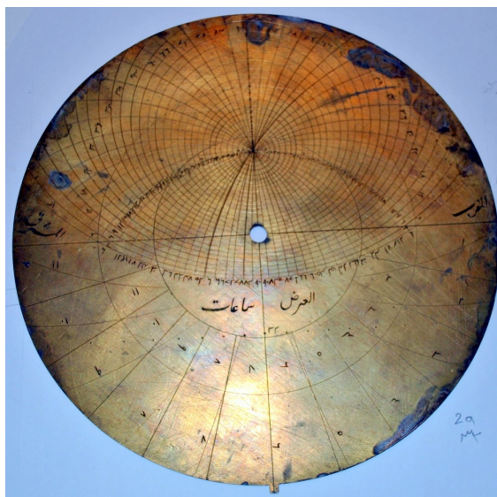
Figure 12: Plate for the Latitude of 32^\circ (photo by Mubashir Ul-Haq Abbasi)
