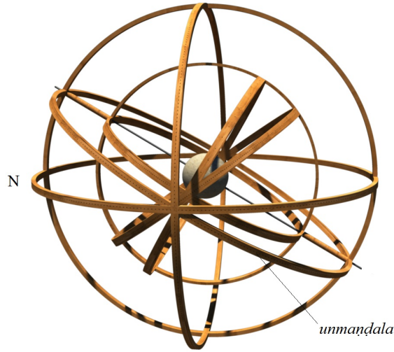
Figure for ¶ 19: Addition of the six o'clock ring ( unmaṇḍala ).
