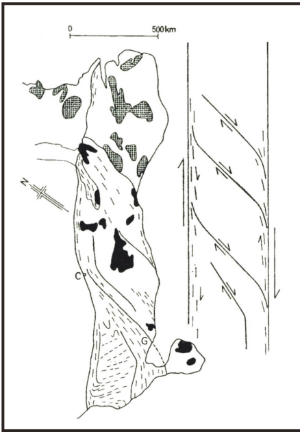
Figure 12. Shear zone model for the Grenville Province (from Baer 1977). Model based on identification of the Chibougamau–Gatineau aeromagnetic lineament (C–G) and its interpretation as a major shear zone. Dashed lines in figure represent regional structural trends; black and cross-hatched bodies are AMCG complexes. Model implies substantial strike-slip displacement along both the Grenville Front, and along approximately N-trending shear zones at high angle to the Front, for which no evidence has been found.
