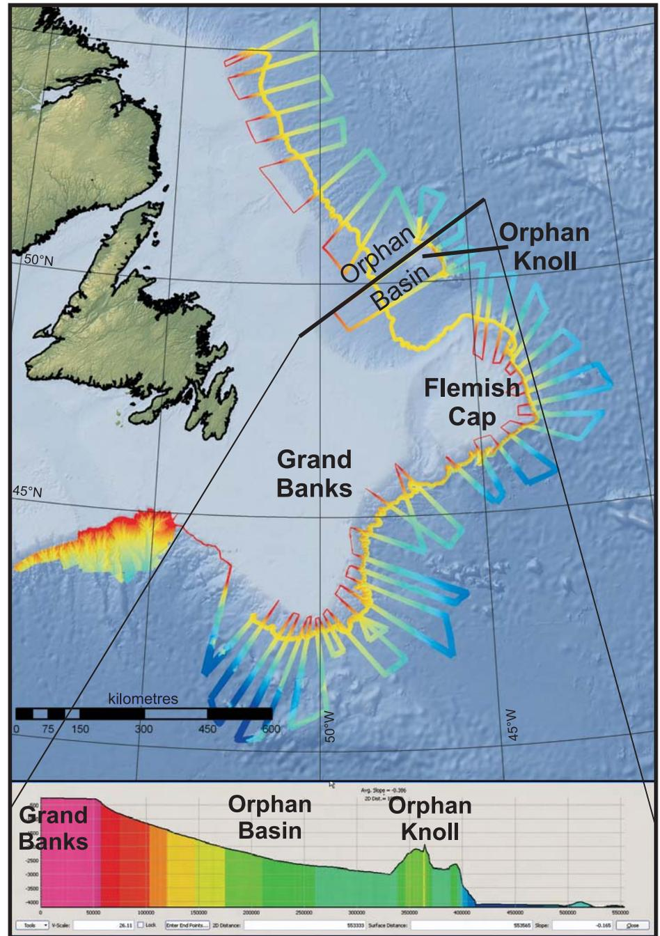
**Figure 6.** Location of the 2006 multi-beam bathymetry profiles around the Grand Banks. Together with existing bathymetry data in the area, these data will provide locations for the FOS. The inset shows a bathymetric profile across Orphan Basin and Orphan Knoll.
