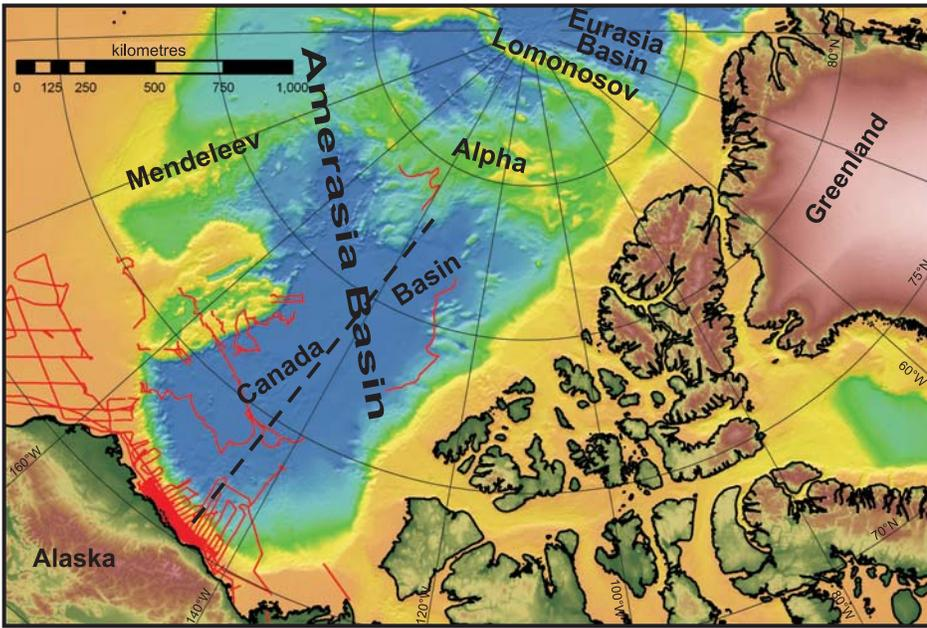
**Figure 8.** General bathymetry of the Arctic Ocean (based on the International Bathymetric Chart of the Arctic Ocean; Jakobsson et al. 2003). Also shown are the main structural features as well as seismic data (red lines) in and around the Canada Basin that were collected prior to Canada's ECS surveys. The dashed black line is the approximate location of the seismic profile shown in Figure 12.
