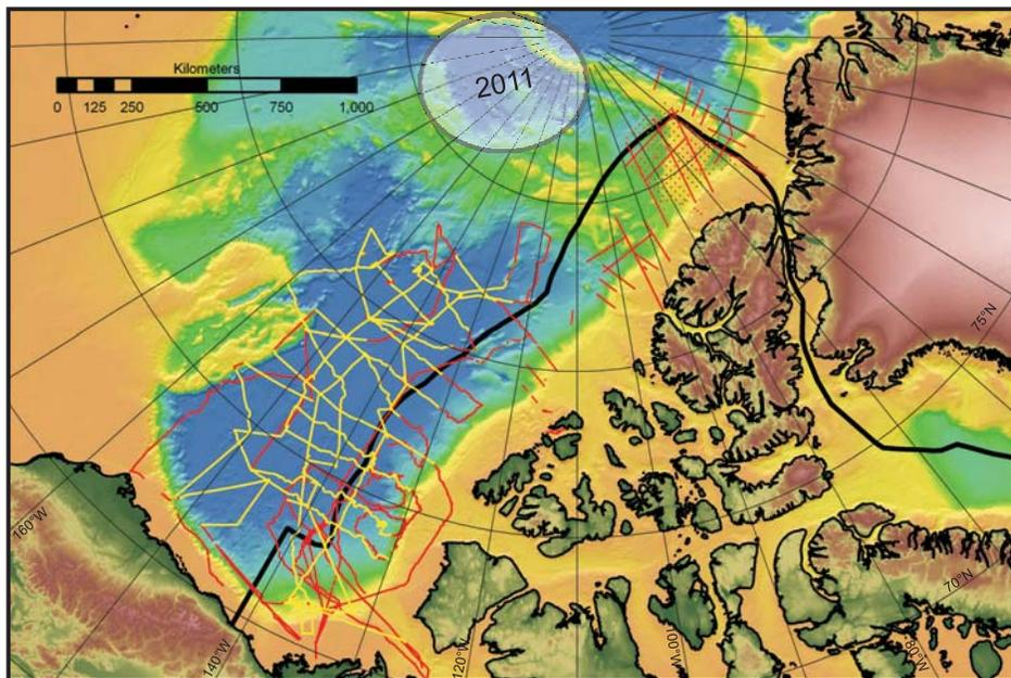
**Figure 11.** Overview of seismic (yellow) and key bathymetry (red) data collected over the period 2007–2010 in the Arctic Ocean. A total of over 13 500 km of seismic and over 18 000 km of bathymetry data tripled data holdings in the Arctic. Also shown is the outline of the area for the 2011 survey.
