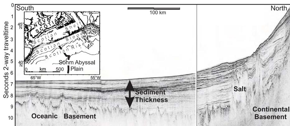
**Figure 4.** Example of a composite of seismic lines across the Scotian margin into the Sohm Abyssal Plain (see inset for location). This record clearly shows the large thickness of sediments extending into the abyssal plain.
