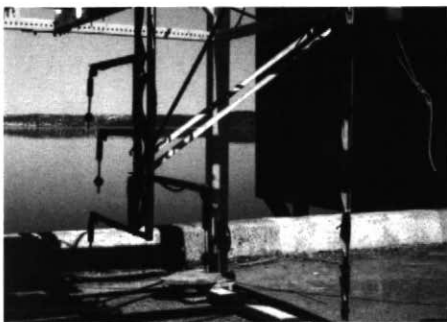
Figure 3 Photograph showing the EMCM array (black balls, on the left portion of the photo) and the OBS array (on the vertical triangular frame, right portion of the photo) that are mounted on the GSC instrumented platform RALPH.
