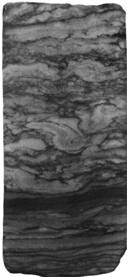
Figure 7 Deformed (slumped?) laminated to thin-bedded anhydrite which can easily be confused with displacive nodular anhydrite. Ordovician (Herald Fm.), Saskatchewan. Core is 10.5 cm across.
