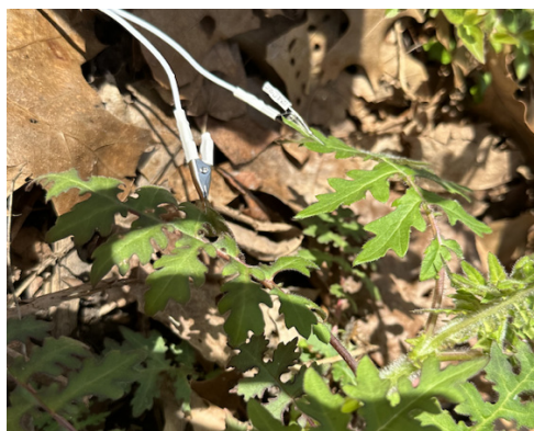
Figure 1. Electrical impulses of ephemeral plants were recorded and converted to beautiful sounds that were played in recessed alcove listening stations along the northside corridor (see Figure 2)
