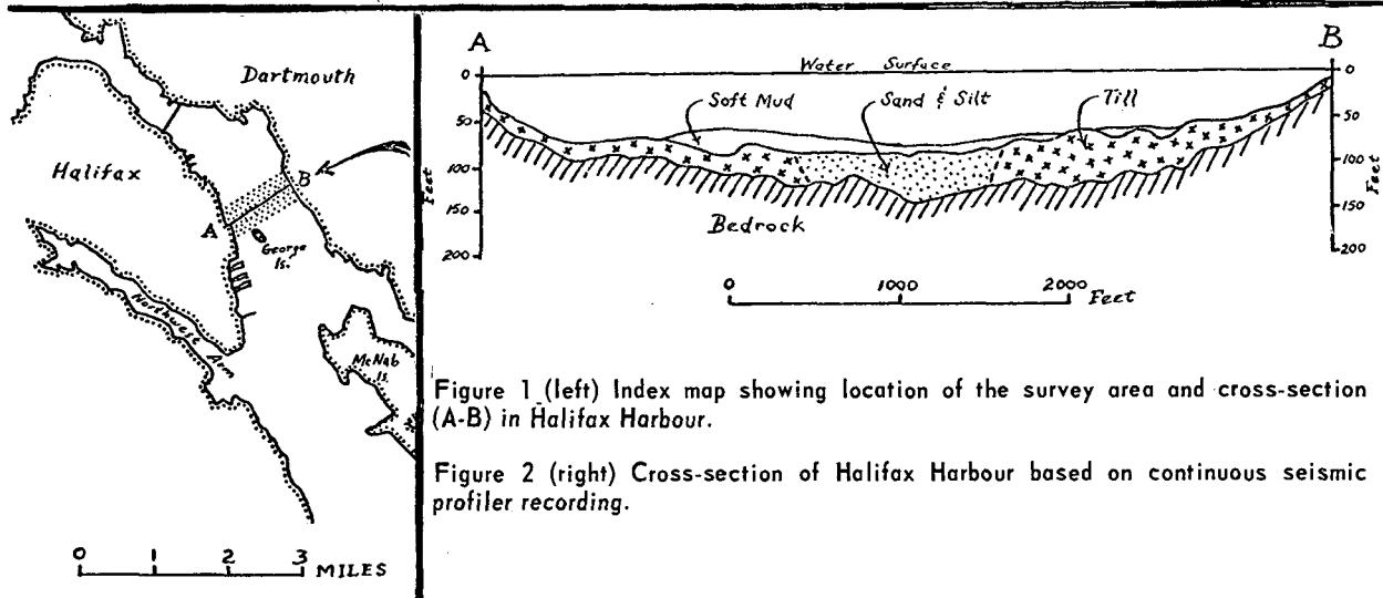
Figure 1 (left) Index map showing location of the survey area and cross-section (A-B) in Halifax Harbour.
