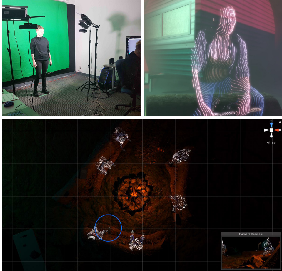
Volumetric capture with greenscreen, in-game preview and overhead view of a 3D scene in Unity. Images produced during the making of the VVV project. See database entry.
