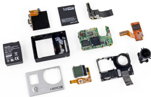
Components of the GoPro HERO3 (2012). See database entry.
