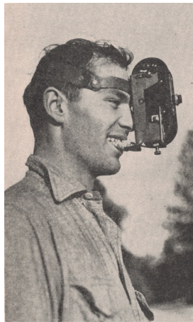
8 mm camera modified to be worn on one's head and used hands free.
