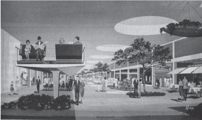
FIGURE 6: Victor Gruen's proposal for a pedestrian concourse below street level in which people movers are located at single-story height within a skylit double-height subterranean space.
