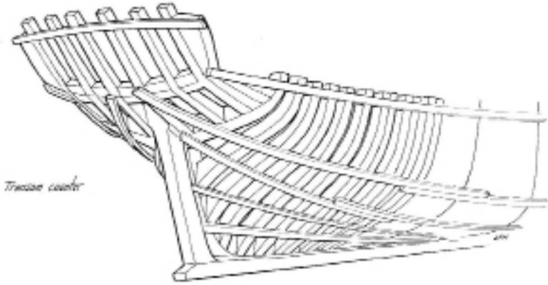
Figure 20. Framing of the transom counter of a nineteenth-century schooner.
