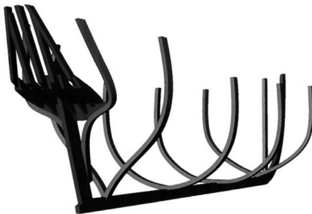
Figure 13. Keel of Indeavour showing structure of counter and frames of the main stations, as drawn by author.
