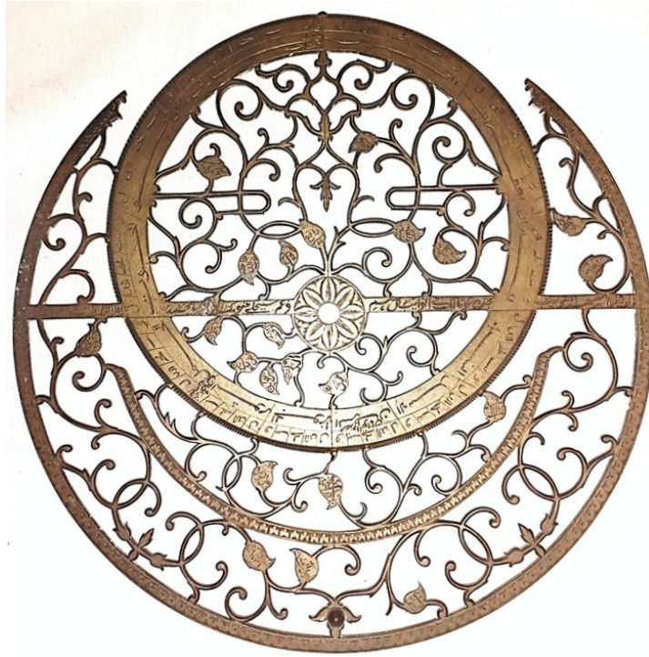
Figure 5: Rete of the Astrolabe (photo by Mubashir Ul-Haq Abbasi).
