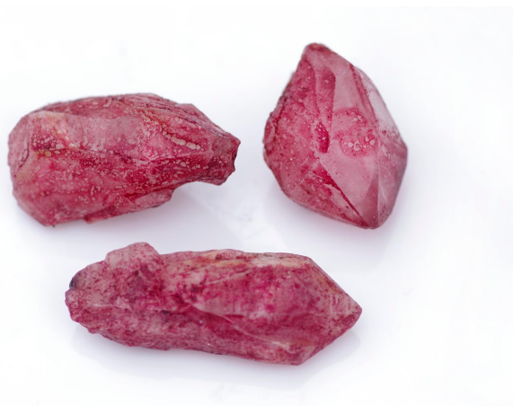
Figure 3: Quartz crystal dyed with fish black and coated with mahua oil. © Andrew Mason.
