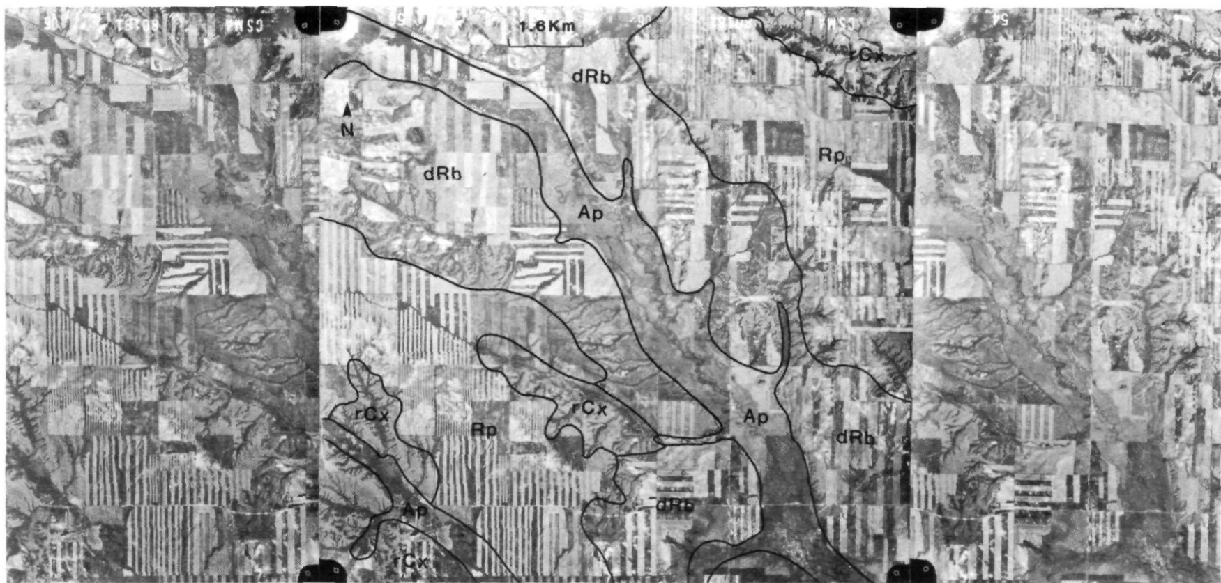
FIGURE 9. Stereo-triplet of southeast part of Wood Mountain area, showing unglaciated bedrock (Rp), gentle slopes (dRb), and alluvial plains (Ap) of Poplar River valley (centre) and Bolster Creek (left corner). Centre of figure is Sec. 22, tp. 2, rge. 1 (49°08'N, 106°04'W). Airphotos CSMA 80181-06-12-54, 56, 58.
