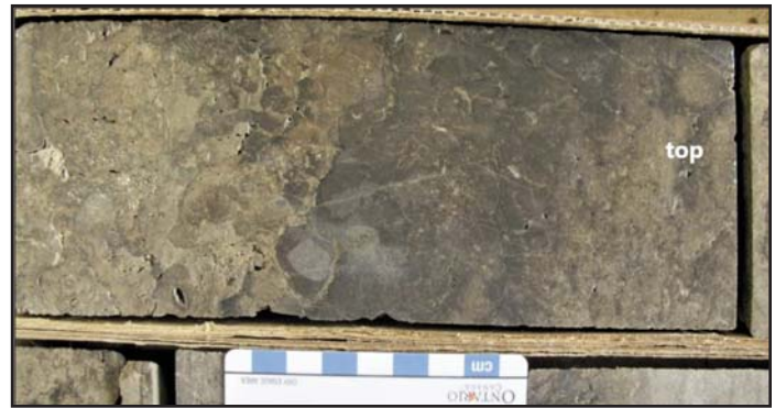
Figure 22. Dark brown to black, dolostone paleokarst rubble in the inter-pinnacle Guelph Formation, 800.5 m below rig floor. Drill core from petroleum well Tec. Dow 4, Moore 21-XII, in Lambton County, well licence #T007290, core # 996 at the OGSRL. This paleokarst rubble forms a regional brine aquifer in the regional karst and inter-pinnacle karst belts in southern Ontario.
