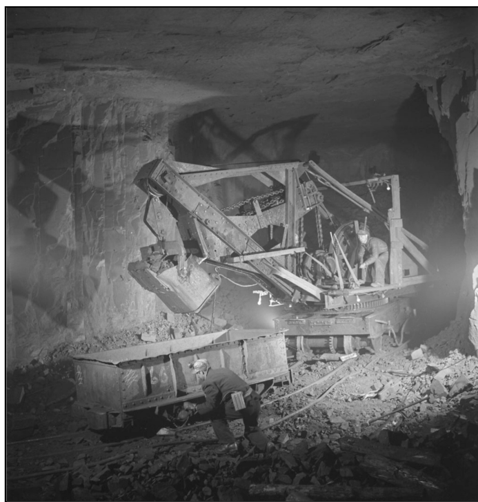
Figure 16. Electrically-powered mining shovel loading ore in No. 3 mine, August 1949. Photo by George Hunter. Courtesy of Library and Archives Canada (PA-4948444).
