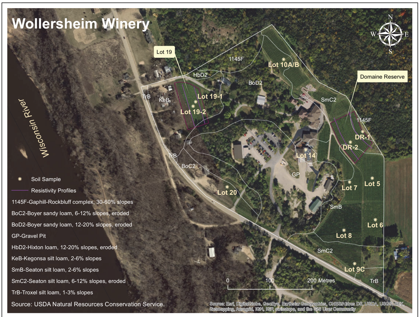
Figure 4. Location map of Wollersheim Winery vineyards illustrating the distribution of soil types, and soil sample and resistivity profile locations.
