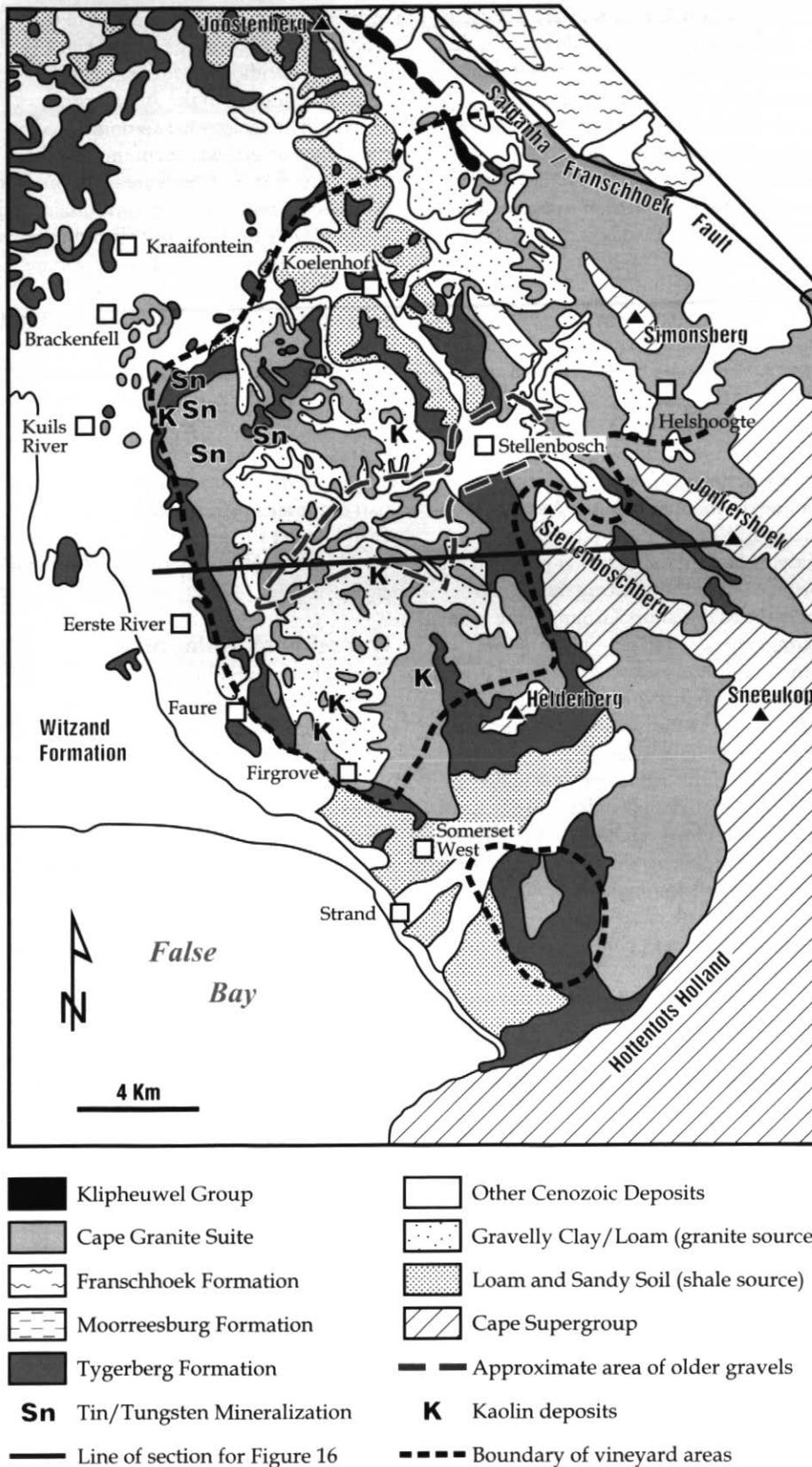
**Figure 18** Generalized geology of the Stellenbosch District and the Joostenberg area, Coastal Region of South Africa. Line in centre of figure indicates location of schematic east-west cross-section seen in Figure 16. Modified from Geological Survey of South Africa (1990).
