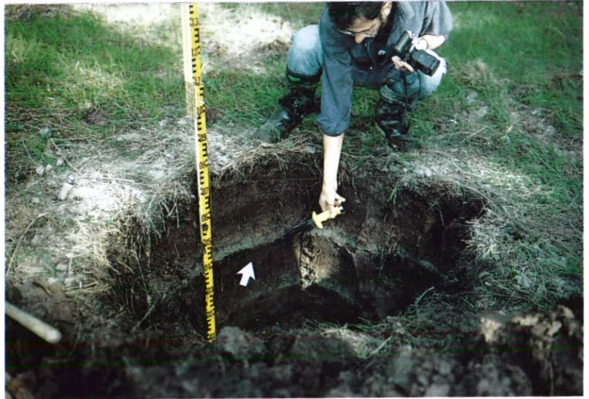
Figure 6 Buried peat layer (arrow) exposed in a pit dug in a tidal marsh near Tofino, British Columbia. The peat layer delineates a former marsh surface that subsided about one-half metre during the last great Cascadia earthquake 300 years ago. The peat is overlain by a thin layer of sand (tip of knife), deposited by the tsunami that followed the earthquake. The sand, in turn, is overlain by tidal mud (photo by J.J. Clague).
