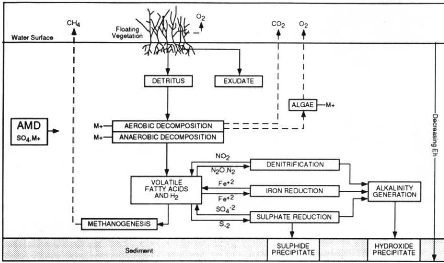
Figure 5 Macrophyte-based wetland system for remediation of acid mine drainage (AMD) showing principal biogeochemical processes.
