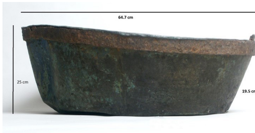
Figure 6. Dimensions of the copper kettle (MAUM: 51.4.15)
