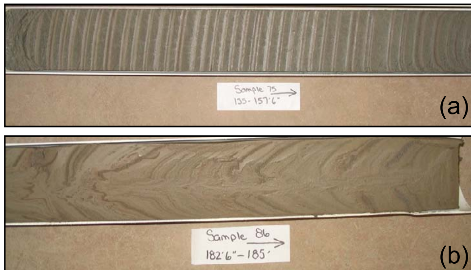
Figure 7. Examples of split cores in ~60 cm (2 ft) lengths from a depth of approximately 47.3 m (155–157.5 ft) below surface, demonstrating (a) finely laminated silt and clay, and (b) fluid deformation of core from a depth of approximately 55.7 m (182.5–185 ft); core diameters are 73 mm wide and arrow points towards top of core.
