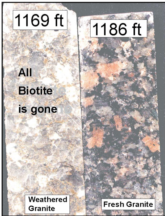
Fig. 15. Photographs of the paleosaprolite and parent unweathered granite underlying the Horton Group from a drill hole 4 km east of the Three Mile Plains area. Note that the granitic texture is intact; however, all of the feldspar grains are altered to kaolinite and biotite has been completely weathered out.
