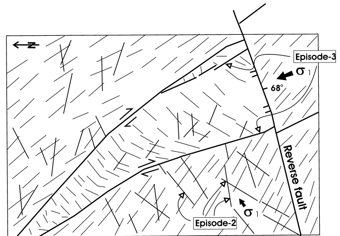
FIG. 8 Episodes 2 and 3 conjugate faults in Flume Ridge phyllonitic metasedimentary rocks in Kellyland zone. Line drawings from photography. Northeast side of Third Machias Lake.
