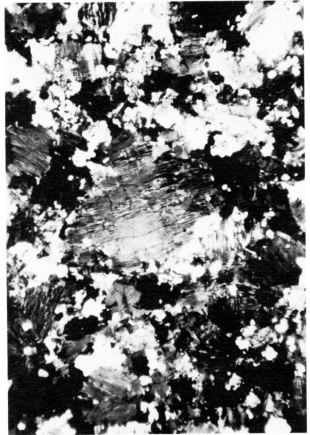
Fig. 6. Photomicrograph of charnockitic syenite from the Cormacks Lake complex. Note the large string mesoperthite grains, interpreted as original igneous grains, surrounded by finer-grained mosaic feldspar and quartz. Minor orthopyroxene, augite and hornblende also occur in the slide. Size of field 3.1 x 4.5 mm.
