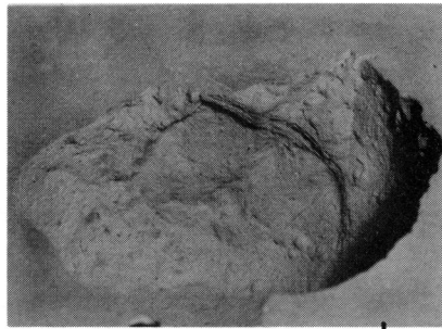
Fig. 6 - (Stereopair). Striated groove cast on the roof of an experimental mud intrusion.
