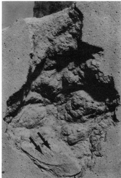
Fig. 7 - (Stereopair). Inward-bulging load-structures on the walls of an experimental mud intrusion. A mass of cement, intercalated with mud laminae (arrowed) probably formed by repeated slumping of cement from the walls during mud intrusion.
