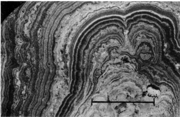
Fig. 5 Detail of alternating lamination of Type A morphology. Photonegative of a thin section. Scale bar 10 mm.
