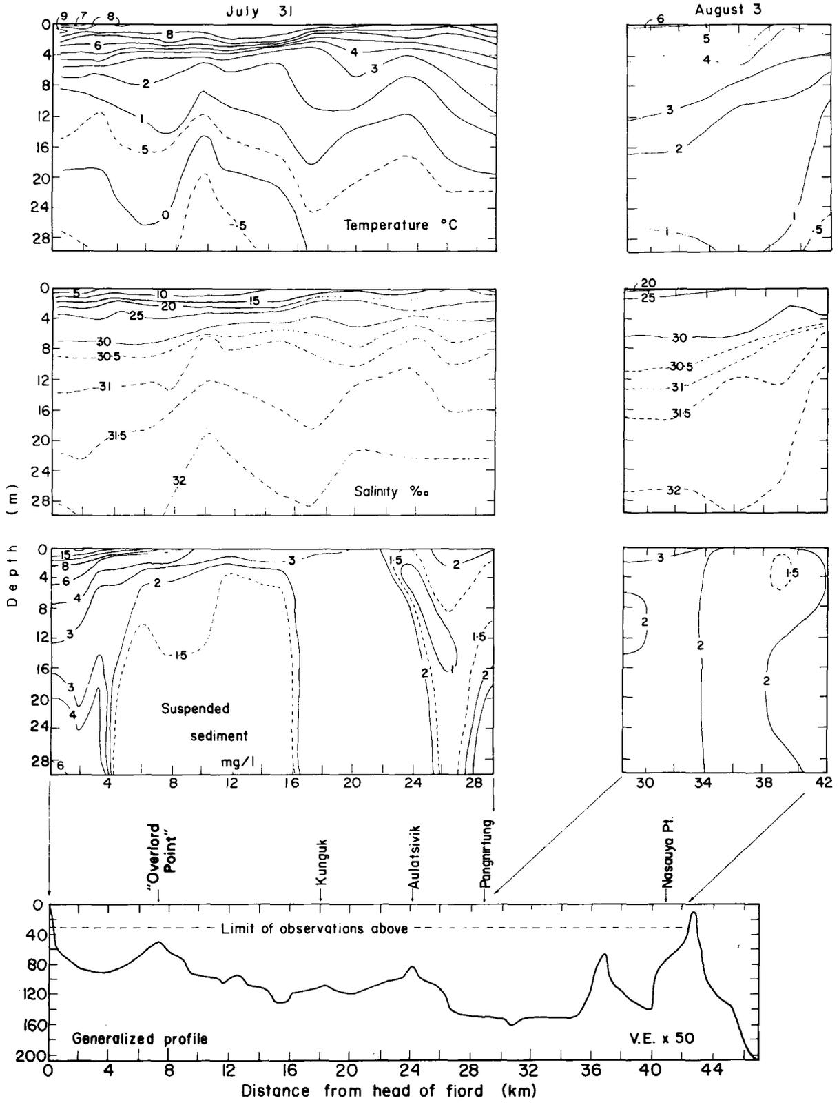
FIG. 3 Temperature, salinity and suspended sediment in the upper 30 m of Pangnirtung Fiord. Transmissivity of incandescent light was calibrated against dried residue retained on 0.22  $\mu$ m filters from samples taken beside the probe near the surface. Measurement stations were located at 1- to 2-km intervals along the fiord.
