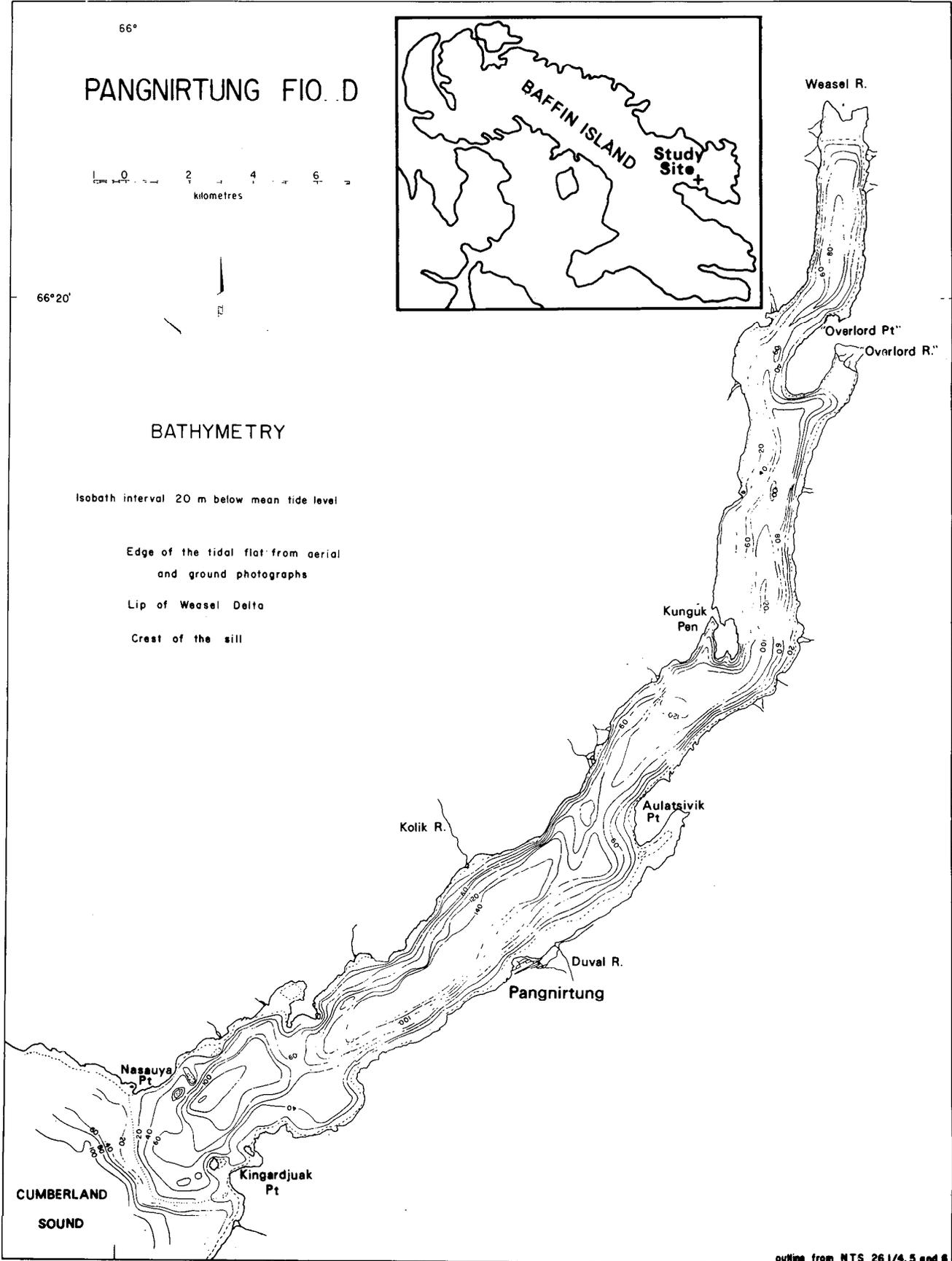
FIG. 1 Bathymetry of Pangnirtung Fiord. A conventional echo sounder was operated on transects across the fiord at 0.5- to 1-km intervals, and down the length of the fiord. Positions were determined by line-of-sight to points recognisable on aerial photographs. Depths are below mean tide level based on water levels recorded at Aulatsivik Point. Names in quotation marks are not officially recognised.
