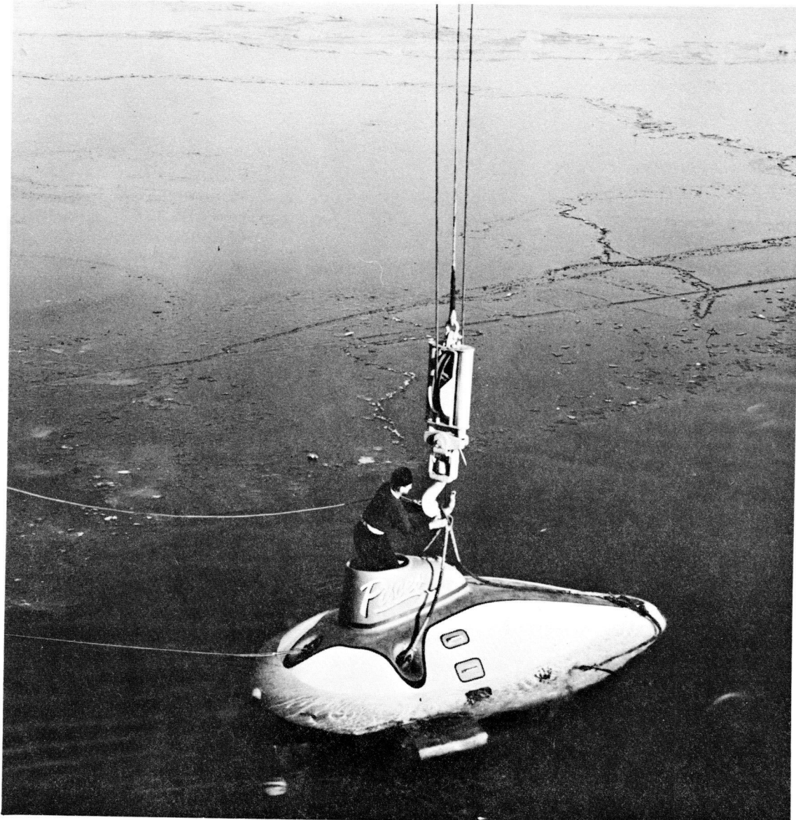
Figure 4 Submarine operator standing on closed hatch and unhooking crane prior to submerging. Photo by Dept. of National Defence.
