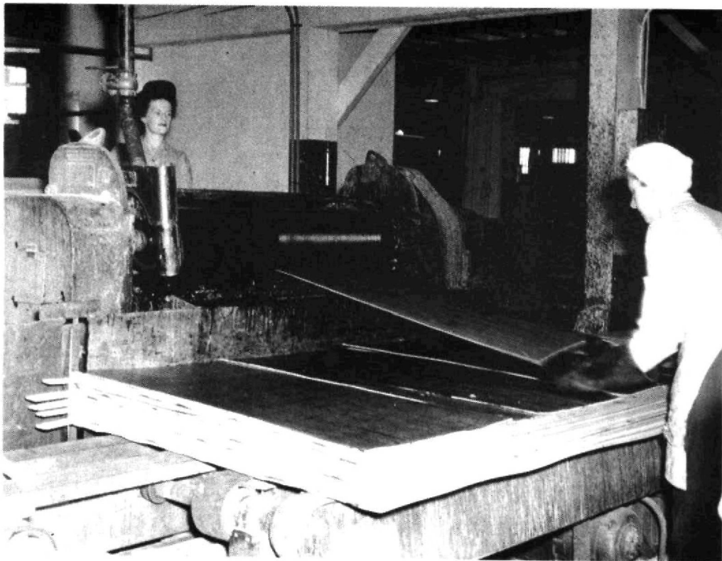
Figure 3. A female core-layer (right) pulls freshly-glued core out of the gluer. Next she will set it down onto the veneer, and another sheet of veneer will be placed on top. Afterwards, the layers will be pressed together in a hot press. Plywood consisted of three, five or seven layers of veneer and core. C.1944.
